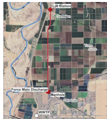
Force Main from Lift Station to WWTP
